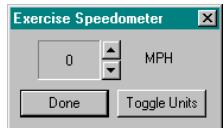
While the tool is in the exercise gauge mode, it will continuously broadcast ATA data link messages to simulate an engine or a vehicle operating condition. However, this mode is only useful if the instrument panel cluster that is under service has been programmed to operate from the ATA data link. No other tool feature is made available until the exercise gauge mode is complete by clicking on the button.
